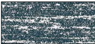
Original HSS-milling cutter • brittle construction • limited strength
