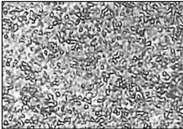
Finegrain-hardmetal structure Ultra-micro-grain, grain size 0–0.5 micron
